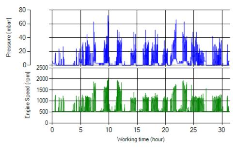
Figure 14- P, N distribution vs. working hours
