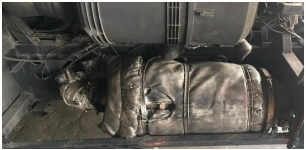
Figure 1. Unsuitable filter isolation
