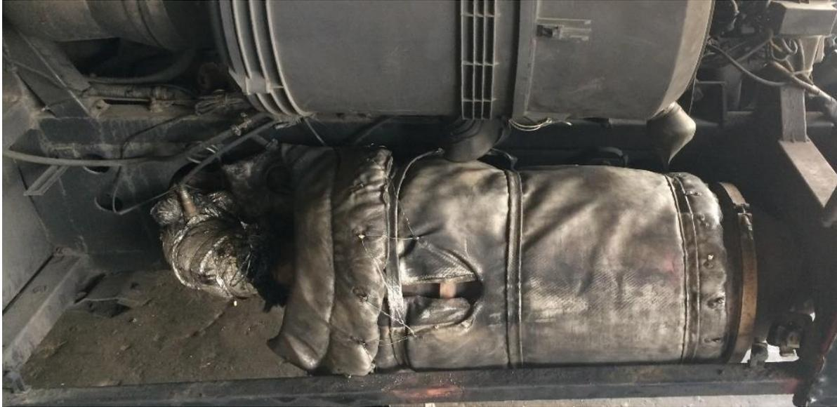
*Figure 1. Unsuitable filter isolation*
