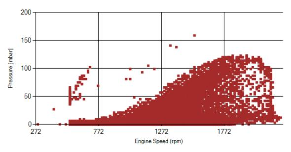
Figure 11- Pressure against engine speed
