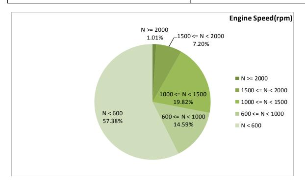
Figure 3- Engine speed distribution over the working hours
