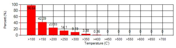
Figure 17. Cumulative diagram of exhaust gas temperature
