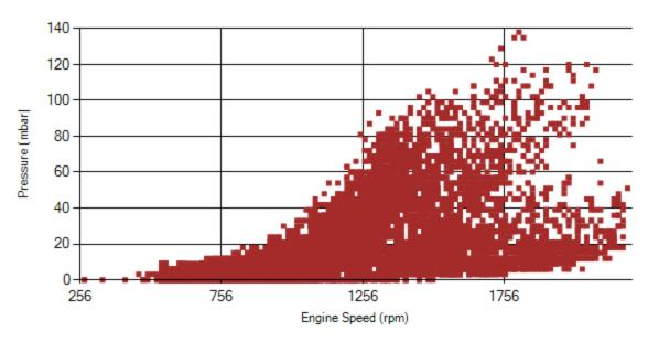
Figure 13- Pressure against engine speed
