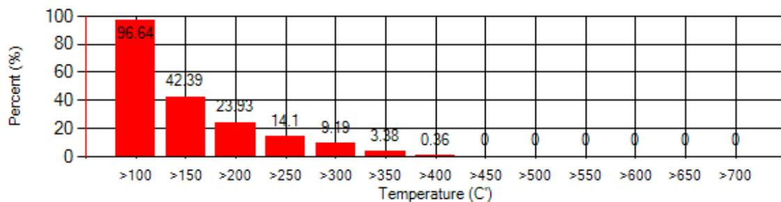
Figure 17. Cumulative diagram of exhaust gas temperature
