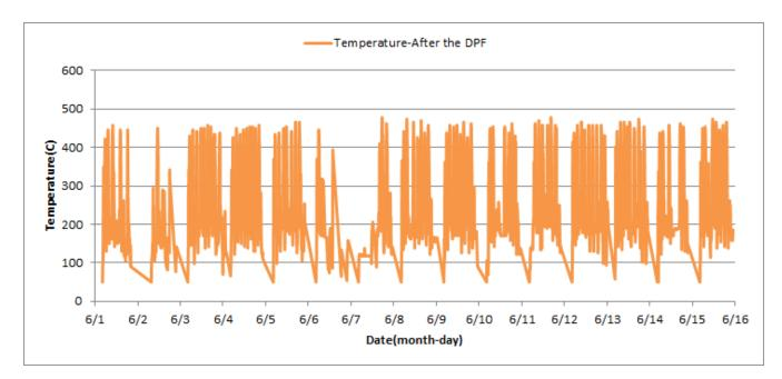
Figure 7- Temperature distribution over the fifteen days
