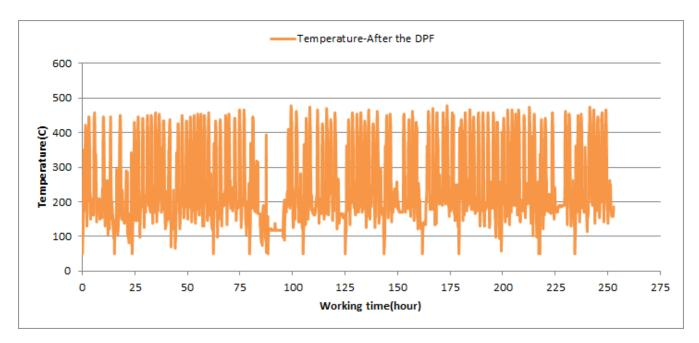
Figure 9- Temperature vs. working hours
